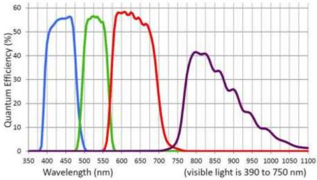
This way is applicable if only two cameras coexist. No additional setting for the software, just install two different wavelength ToF products.
